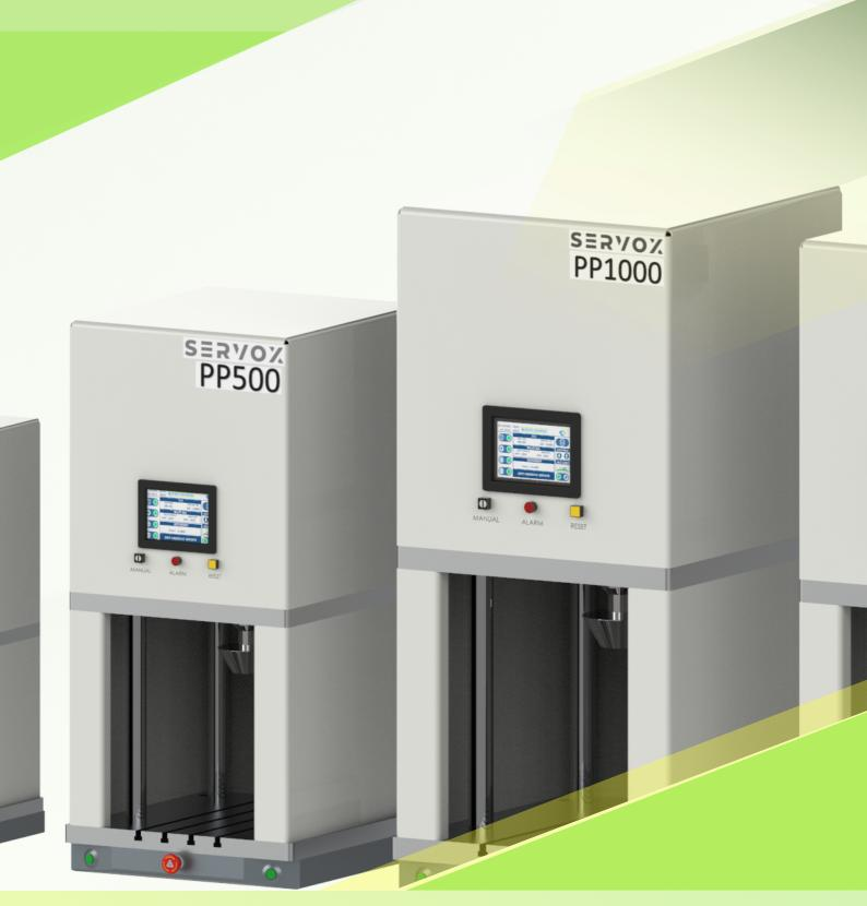
A Servo press consists of a simple rigid structure on which is mounted a die shoe or slotted plate for holding the bottom half of a die. On the frame is mounted a sturdy ball screw driven cylinder which provides up and down movement to the other half of the die. The cylinder is driven by a servo motor and drive controlled by a Plc to control the force, speed, and position of the pressing plate.
